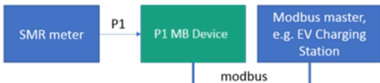
DSMR 4.x does not contain the Voltages found in obis-codes 32.7.0, 52.7.0, and 72.7.0 (L1, L2, and L3) for this case the obis code cannot be empty. That's is why you need DSMR 5.0 protocol or higher, Instantaneous voltage L1, L2 and L3 are available and these are the registers the EV charger uses.
