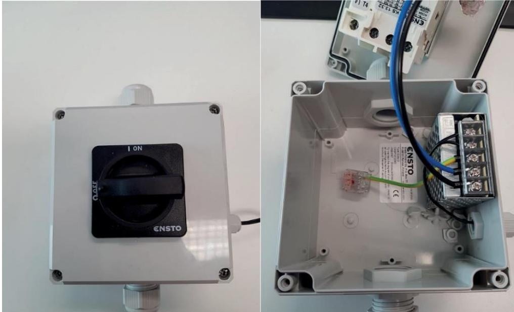
Inside the isolator switch are the transformer and the power cable (1.5m) for the SUNGATE. It also contains the Ensto load breaker switch type KS 13.32, which is an EN 60947-3 certified load breaker switch (3x 32 A), with a maximum cut-off current of 6 kA.
