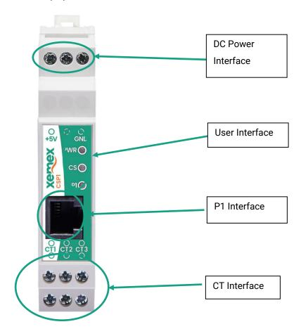
The CSP1 measures the RMS current values of the three current transformer inputs over a period of 1 second.
